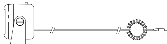
Figure 8. Power lead suppression.
