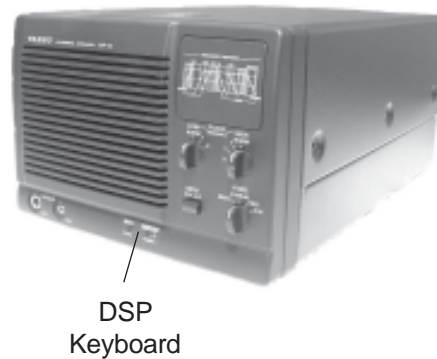
Figure 20. NEDSP1062-KBD installed in a Yaesu SP8.
