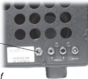
Figure 20. NEDSP1062-KBD installed in a Yaesu SP8.
