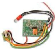
Fit the bhi NEDSP1061-KBD DSP noise cancellation in your Transceiver - Features 4 filter levels with visual and audio indication - Single button operation - Supplied with mounting hardware - Size only 35mm x 26mm - Module will fit most transceivers/receivers. Fitting instructions available for the following radios:
