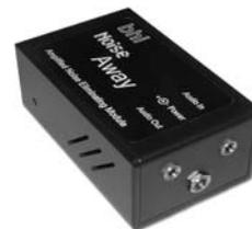
The bhi ANEM "Noise Away" (Amplified Noise Elimination Module) is a compact, microprocessor controlled in-line DSP noise canceling module - Fits in-line between the radio and the loudspeaker - Simple two button operation: power on/off audio bypass and DSP filter on/off - 4 or 8 filter levels - last selected filter level remains in memory. Supplied with a 1030-FPL fused DC power lead & an ALD-001 3.5mm plug lead 1.2 M long.
