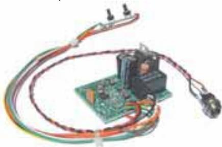
Easy to fit bhi amplified DSP noise cancellation module - Retrofits inside any suitable extension speaker or radio - Features 4 or 8 filter levels - Power on/off with bypass - 2 Watts output - Power connector - Labels - Fused DC power lead - General fitting instructions plus fitting guides for the Kenwood SP31 & Yaesu SP8 extension speakers. Supplied with full fitting kit, labels and fused DC power lead.
