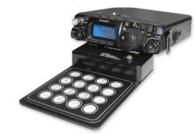
The Radio Mate Compact keypad for the Yaesu FT817, FT857 and FT897 enables the user to get the best out of their radio. It has been designed to make many of the common functions quick and easy to use. The keypad does this with a number of fast, effective shortcuts.
