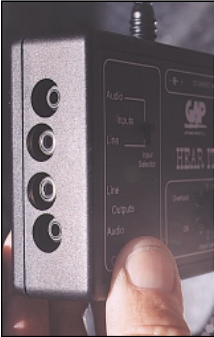
Photo D— Audio input and output cables plug into the side of the “Hear It” module. There are audio-level and line-level connections for both input and output.
