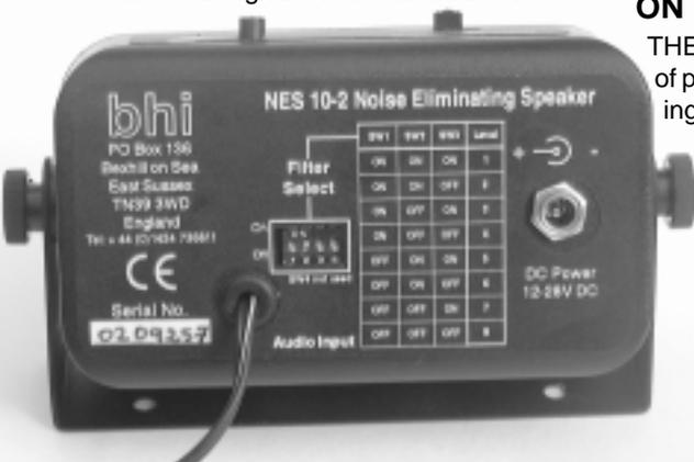
The UK company of bhi, located in Bexhill on Sea, has come up with a very easy-to-use accessory for doing just this. They've incorporated a full-featured DSP noise reduction circuit entirely within a small external speaker casing. Measuring 110 x 65 x 55mm it's the size of a typical compact extension mobile speaker.
