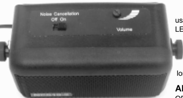
set volume control and a noise cancellation on / off slider switch. The volume control could more accurately be described as a sensitivity control, because once set, I could then use my receiver's volume control as usual to control the overall volume. The speaker gives up to 2.5W RMS output, quite ample for most purposes. A dual-colour LED behind the speaker grille glows red when the noise suppression is off, and green when on, and this illuminates whenever power was applied.
