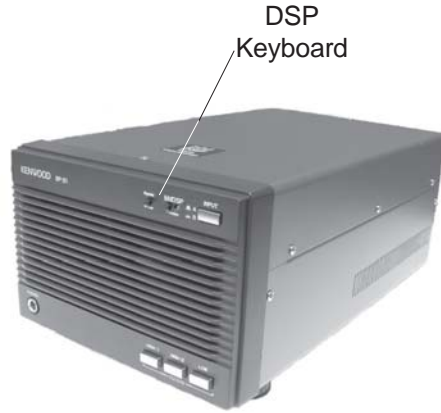
Figure 25. NEDSP1062-KBD installed in a Kenwood SP31.
