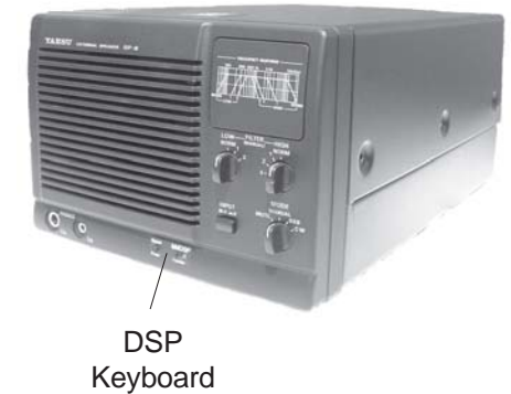
Figure 20. NEDSP1062-KBD installed in a Yaesu SP8.
